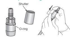
Apply a small amount of the LS OIL or MORITA MULTI SPRAY to the O-ring and shutter of the motor cover, and then slide the motor cover straight onto the micromotor.
