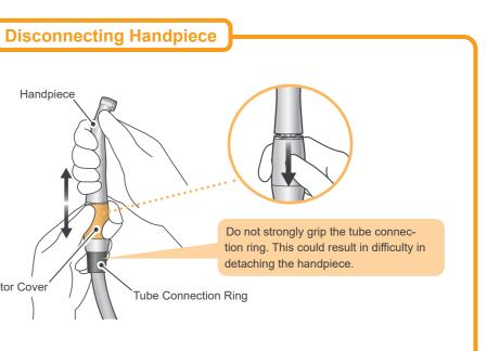
Hold the motor cover firmly and pull the handpiece straight off. (The TORX series has a sliding mechanism the motor cover to disconnect the handpiece.)
