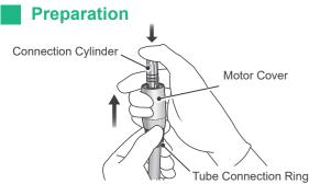
Holding the tube connection ring, grip the motor cover and press down on the connection cylinder with your thumb to slide the cover off the micromotor.
