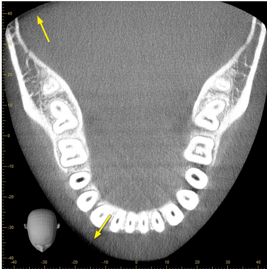
Figure 23: Example of Luminance Degradation in Edge Area of FOV
